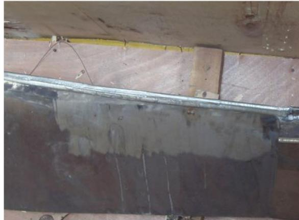
1710mm长叶片边缘激光熔覆Stellite 6涂层
